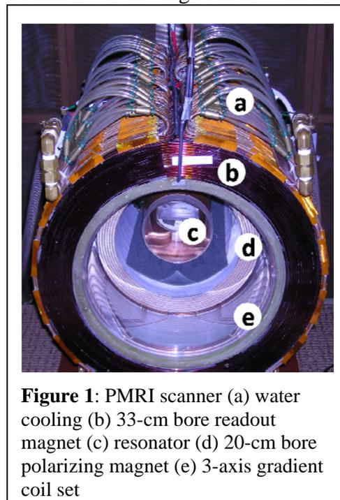
**Figure 1:** PMRI scanner (a) water cooling (b) 33-cm bore readout magnet (c) resonator (d) 20-cm bore polarizing magnet (e) 3-axis gradient coil set
