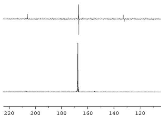
$^{13}\text{C}$  polarized signal before the application of the pulse sequence (above): longitudinal spin order  $I_z^{\text{H}}I_z^{\text{C}}$  is observed, net  $^{13}\text{C}$  magnetization is zero. After the pulse sequence (below) longitudinal magnetization  $I_z^{\text{C}}$  is obtained.
