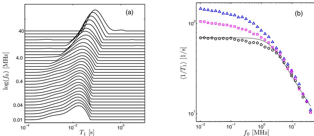
FIG. 1: (a) Evolution of the distribution of  $T_1$  relaxation for a deasphalted crude oil. (b) Dispersion of mean relaxation rates for the deasphalted oil (black circles) and for that same oil with different amounts of dissolved asphaltene (squares and triangles).
