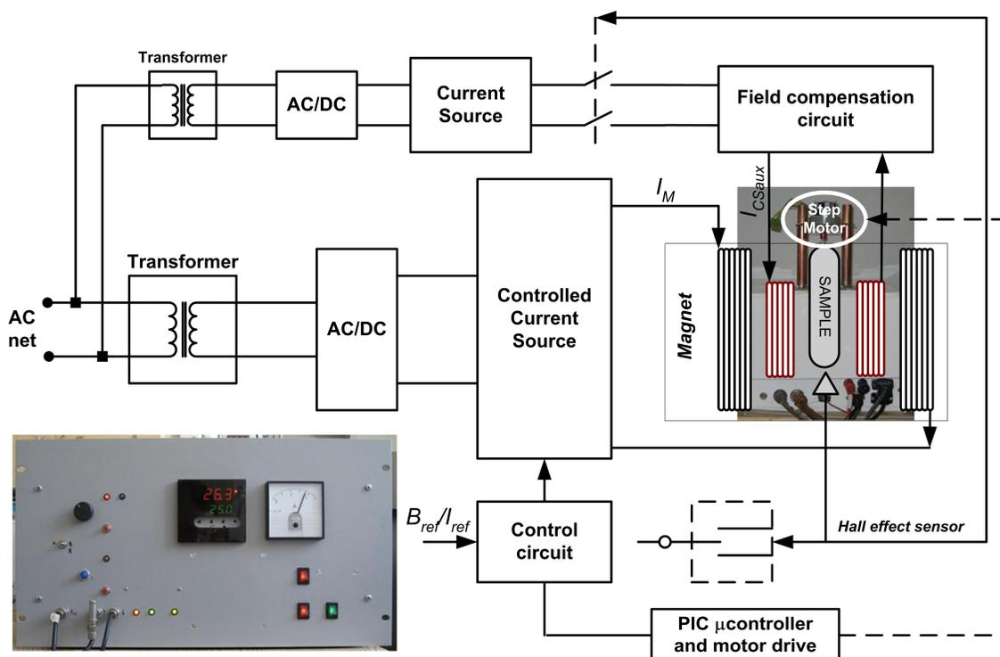
Figure 1 - Main blocks of the desktop FFC relaxometer
