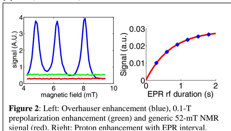
**Figure 2:** Left: Overhauser enhancement (blue), 0.1-T prepolarization enhancement (green) and generic 52-mT NMR signal (red). Right: Proton enhancement with EPR interval.
