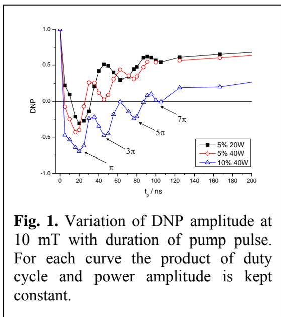
**Fig. 1.** Variation of DNP amplitude at 10 mT with duration of pump pulse. For each curve the product of duty cycle and power amplitude is kept constant.
