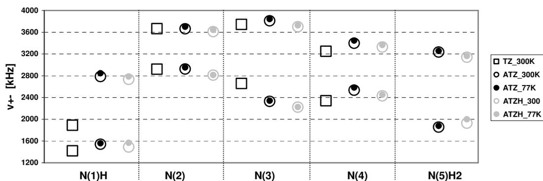
Fig.2. Assignment and comparison of the corresponding  $\nu_+$  and  $\nu_-$   $^{14}\text{N}$  NQR pairs, suitably combined from 1H-tetrazole (TZ, published data<sup>ii</sup>), 5-aminotetrazole (ATZ) and 5-aminotetrazole monohydrate (ATZH) into respective segments N(1)H, N(2), N(3), N(4), N(5)H<sub>2</sub>.
