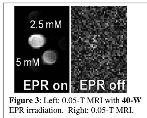
**Figure 3:** Left: 0.05-T MRI with 40-W EPR irradiation. Right: 0.05-T MRI.
